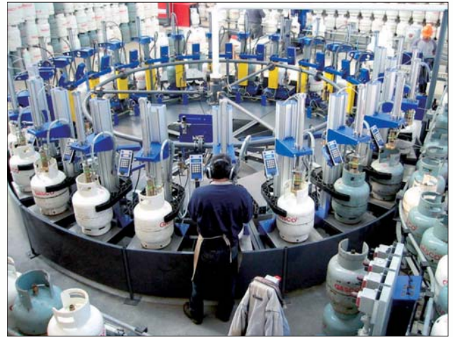
Cylinder filling carousel type EFC/U-24 with 24 electronic filling machines - Also available in smaller models for 8, 12 or 18 filling machines.
